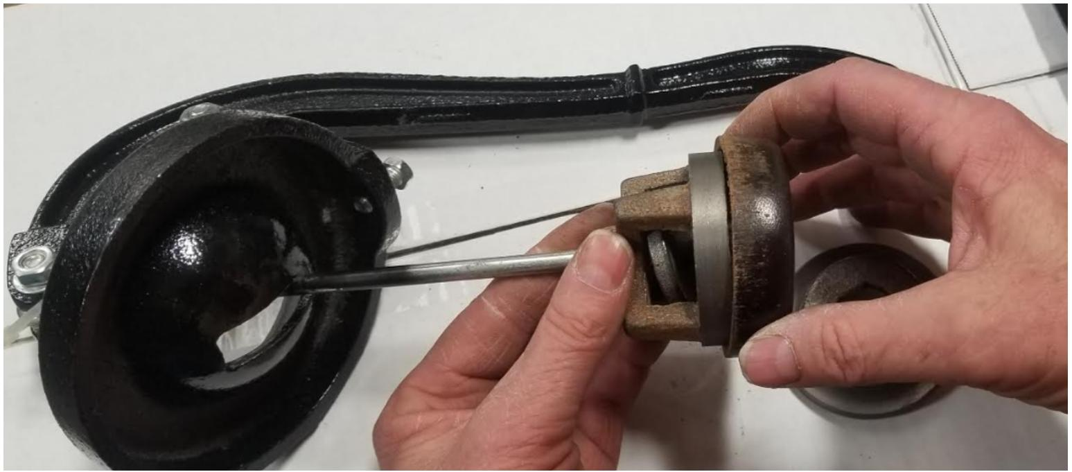
*The above 3 pictures are how to remove the old leather cup to replace it with a new one.*
