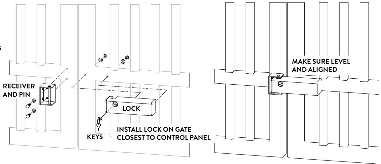
**STEP 4: VERIFY THE RECEIVER PIN LINES UP WITH SLOT IN THE LOCK**
