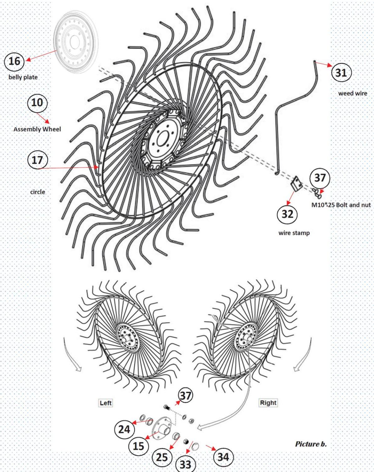
**Note:** Using an overhead hoist or fork lift,carefully tip the assembly in the approximate position it should be in when installed on the tractor and high enough off the ground to install the wheels.Install the wheels on the hubs using the capscrews,lockwasher and nuts the position of the teeth is determined by the direction of operation.
