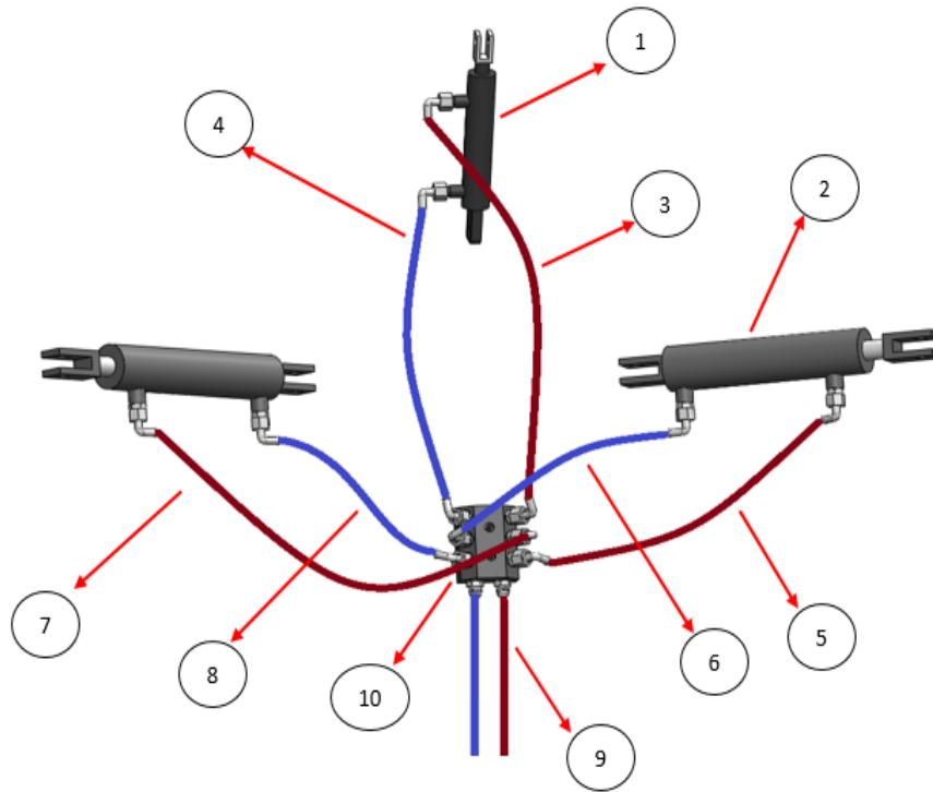
Hydraulic Hoses; Its installation on the hydraulic distributor and hydraulic cylinders must be mounted as shown in the figure.
