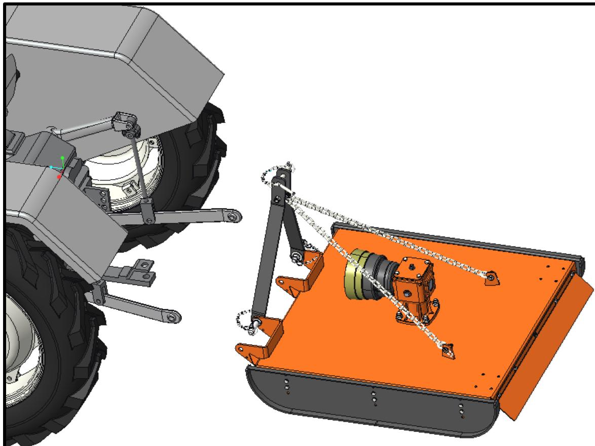
Always work with the driveline as straight as possible. This will prolong life of driveline and that of its components, avoiding premature breakdowns.
