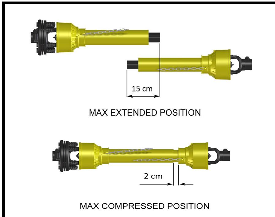
A driveshaft too long may cause structural damages to the tractor and machine. If the driveshaft is too long, it may be adapted by removing it and shortening the tubes according to the instructions provided by the Manufacturer in its use and maintenance manual.
