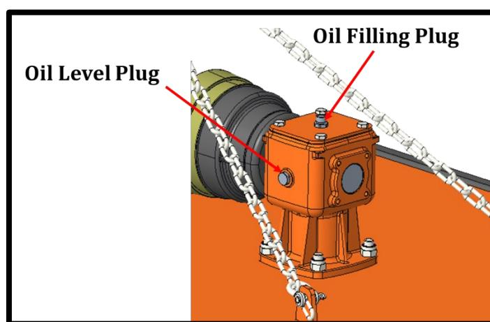
If the mark is below the minimum, fill up oil till restore the correct level.
