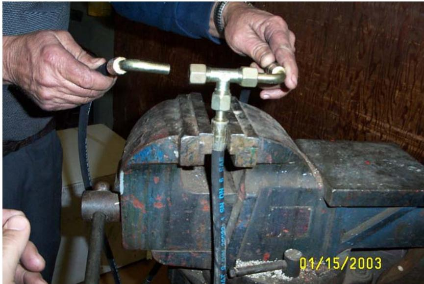
16. Attach the other end of short hoses to the cylinders. Be sure to put brass washer on either side of bolt (19mm wrench).
