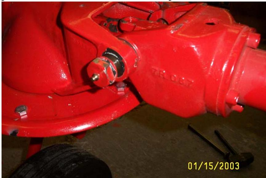
12. Install the outer guard for the unit with the 2 bolts provided in the outer rotor housing- you will need 19mm socket
