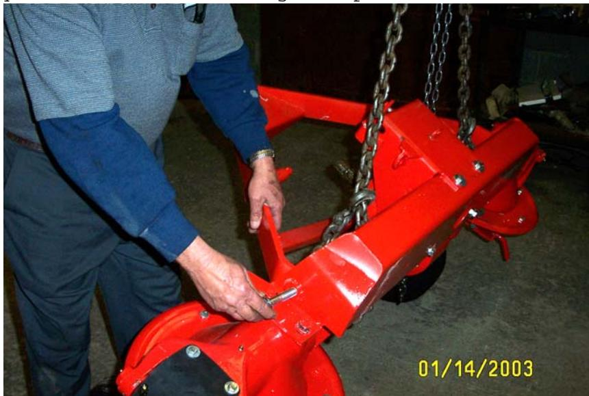
6. Attach the jack stand to the tongue with the cotter key provided in the bag of parts. It is a good idea to grease the jack before installing it.
