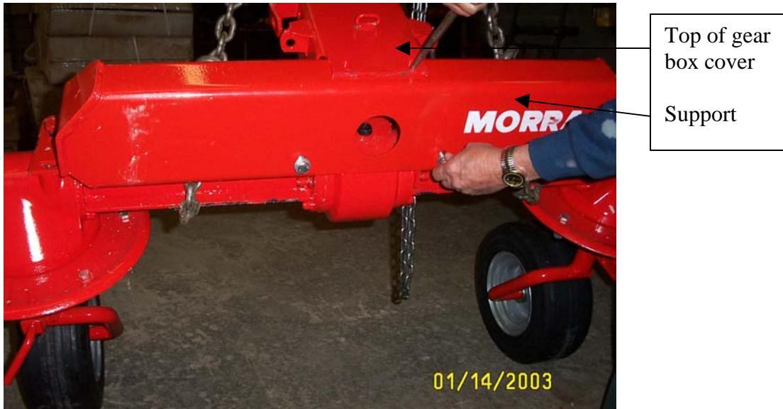
5. Using a 24 mm socket, attach the tongue to the support with the two 8.8 x 80 mm bolts( one on each side) Do not tighten the nuts tightly - you want to allow the tongue to pivot on the bolts.
