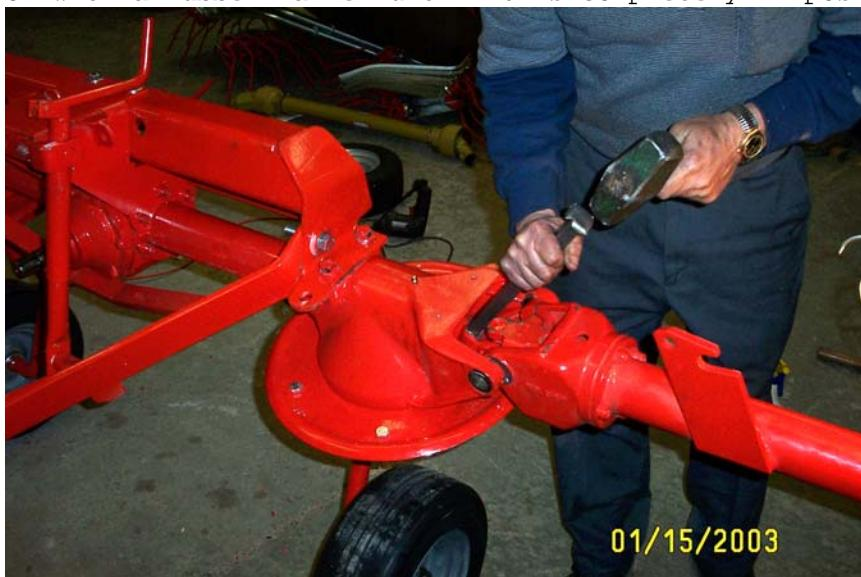
11. Install the grease bolts back in to hold the arm on the unit and place the rubber covers back into place.
