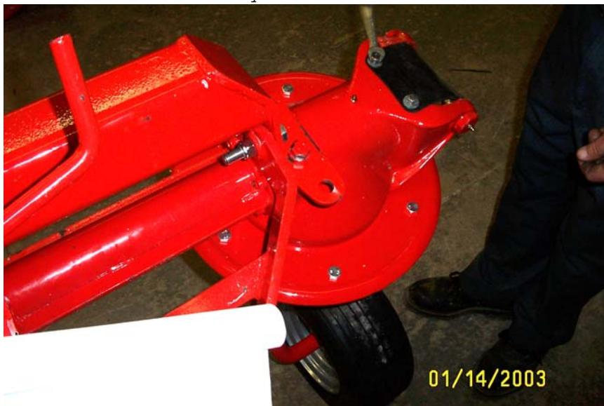
Make sure to remove all paint with emory cloth before attaching the arms & be sure that the grease holes are not clogged. It is a good idea to blow them out with an air gun.
