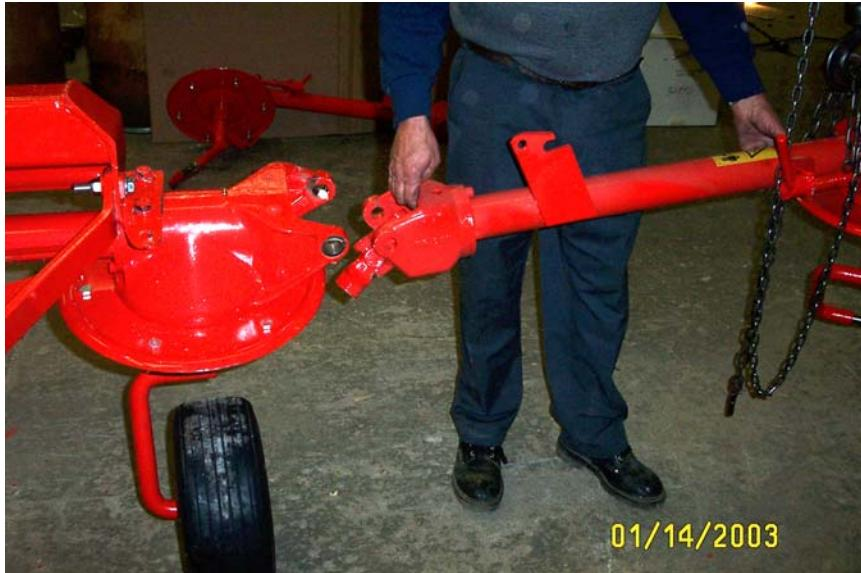
10. To attach the arm to the central unit, turn the rotor on the central unit until the keyway on the shaft is at 12:00 and install the keyway provided. It is also important to be sure there is no paint on the shaft. You will also need to buff the paint from the yokes (inside of central unit, outside of the arm) so that there is no problem with fitting.
