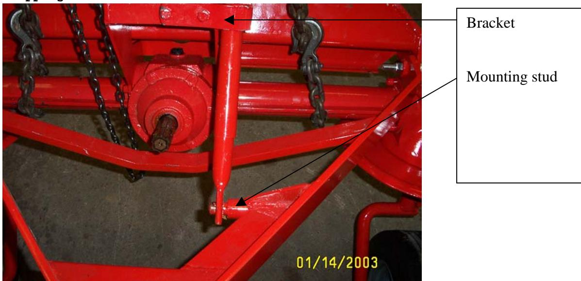
8. Remove the rubber pads with a 13mm socket on each side before attaching the arms to the central unit. Take out the 2 grease able bolts that are in the yokes with a 35 mm socket
