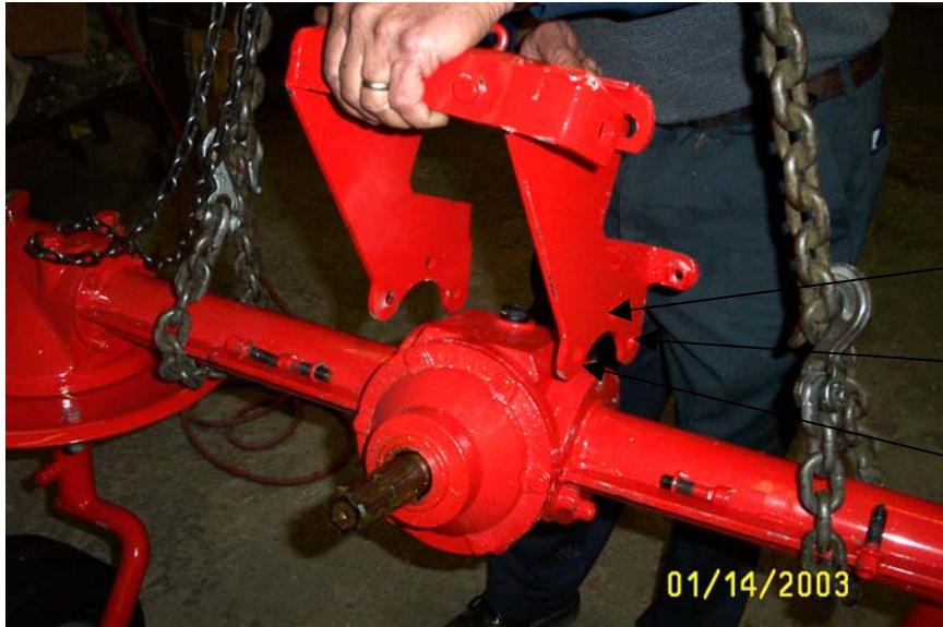
There are three bolt holes on this flange. In this step, only replace front bolt so that it can pivot forward in next step. Then replace other two bolts
