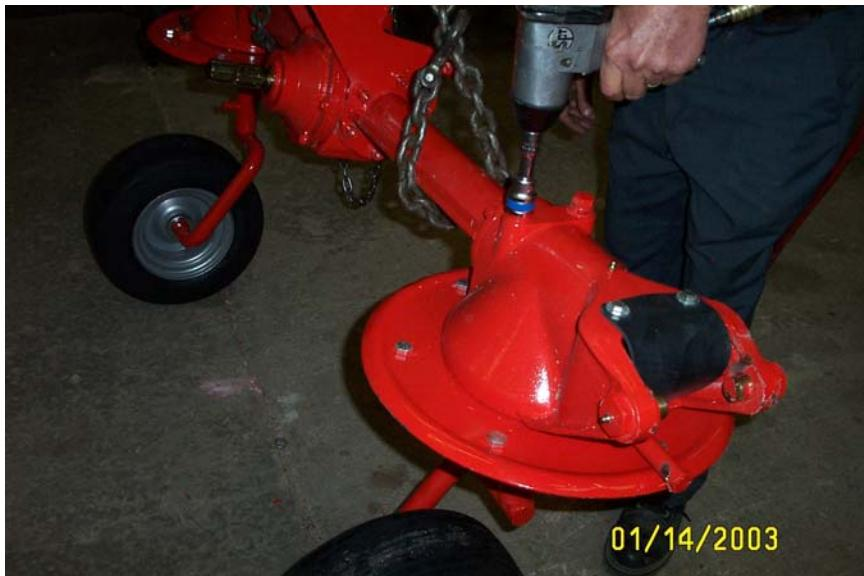
4. Put the 2 bolts back in the flange that goes over the rotor housing. Install 2 bolts and washer in the rear and top that secures the support to gear box cover using a 19 mm socket (top holes are bolt and nut-bottom threads into cover)
