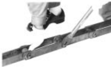
Figure 11-3: Inserting New T-pins or Cotter Pins
