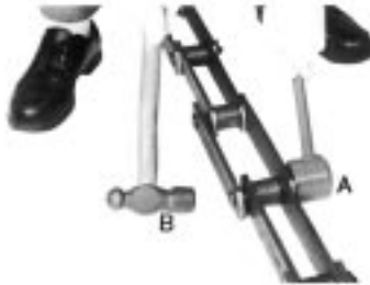
Figure 11-2: Putting on the Link Plate
