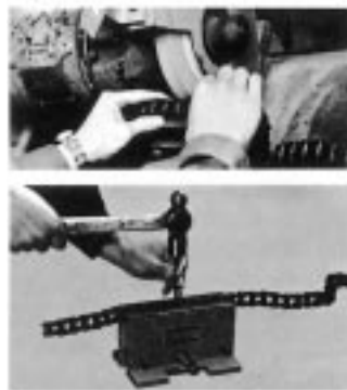
Figure 4-1: Disconnecting RS Roller Chain
