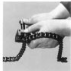
Figure 4-5: Using the Chain Breaker
