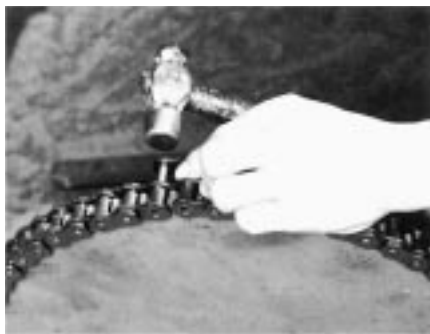
Figure 3-1: Connecting RS Roller Chain on a Sprocket
