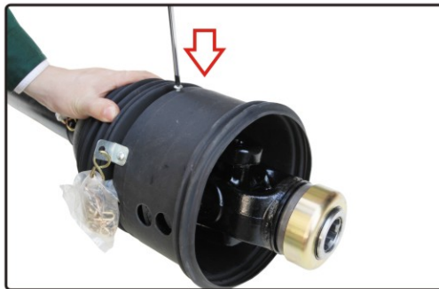
5. Install the screws arranged radially around the circumference of the CV cone.
