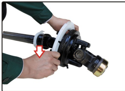
3. Install the bearing ring on the CV boby with the reference pins facing the inner yoke.
