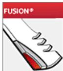
**Stays Sharp Twice as Long** - Using exclusive electrofusion technology, OREGON's Fusion<sup>®</sup> manufacturing process creates an ultra-hard layer at the blade's cutting edge using tungsten carbide, actually embedding it within the blade.
